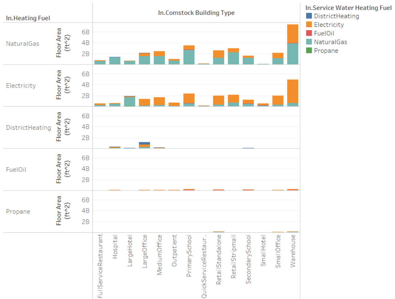
Figure 33. Floor area served by each service water heating fuel by space heating fuel and building type.
